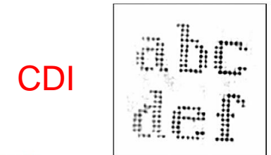
Figure 4 The specimen image as reconstructed from the diffraction pattern of Fig. 2.
